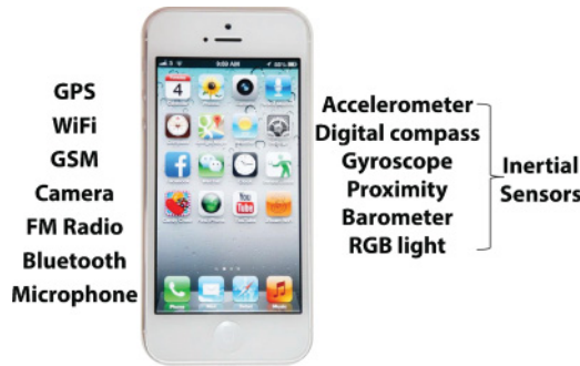
Fig. 5. Candidate sensing modalities on smartphones for indoor localization.
