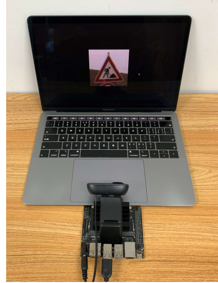
Fig. 6. Hardware setup to measure the execution time of the nine inference tasks (the photo was for the traffic sign recognition task, i.e. , the GTSRB dataset [43]) on the Jetson Nano embedded platform.
