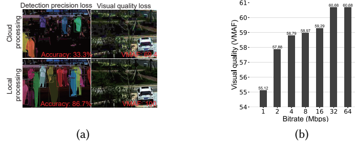
Fig. 3. Comparison of video enhancement locally on-device and remotely on-cloud. (a) Example frames enhanced by local processing and remote processing. The upper row follows the encode-decode-enhance pipeline of remote processing, while the lower row are directly enhanced as in local processing. (b) Enhanced video quality of the encode-decode-enhance pipeline under different frame bitrates into the video codec.
